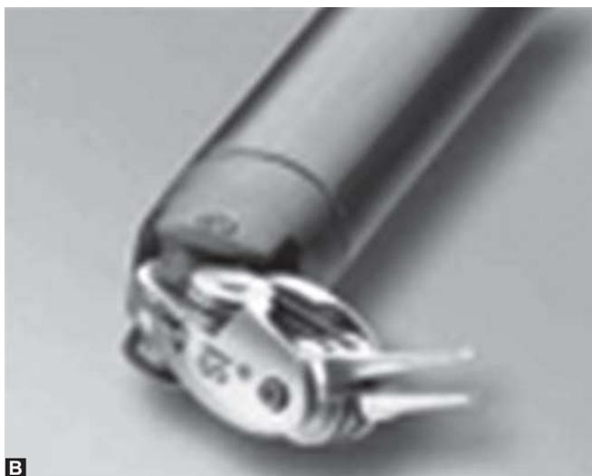
**Figs 2A and B:** (A) New generation robotic instruments have seven degrees of freedom as the human hand, (B) EndoWrist<sup>®</sup> instrument from intuitive surgical (Courtesy: Intuitive Surgical Inc, Sunnyvale, CA)
